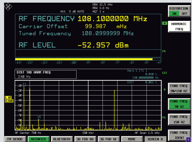
FIG 3 Distortion analysis of an ILS signal. The sum signal derived from 90 Hz and 150 Hz is at 240 Hz, and produces a total harmonic distortion of 0.5 %.
