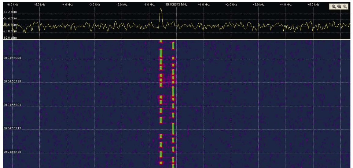
FIG 3 The speed of the spectrum calculation can be set to between 20 and 1000 FFT lines per second. As a result, the waterfall display has a time resolution of up to 1 ms, as can be seen here in the case of a signal with FSK2 modulation and a symbol rate of 50 baud.
